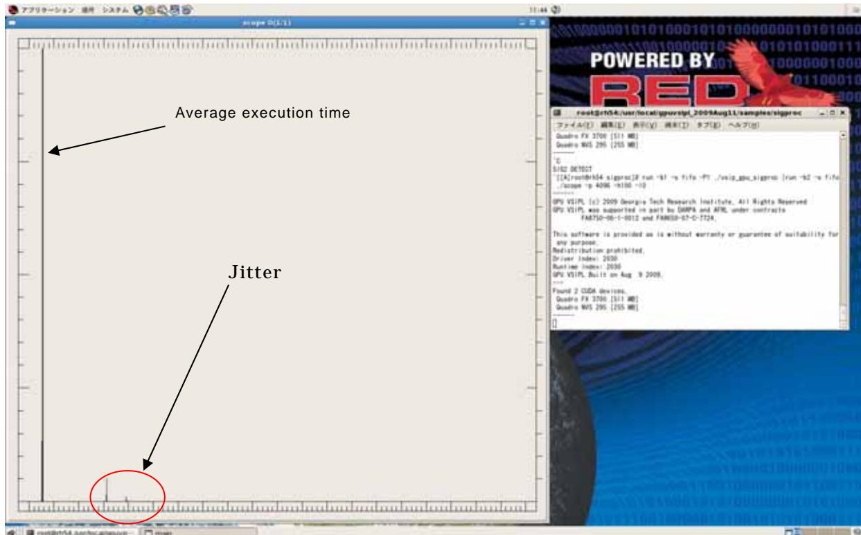
**The result of having run CUDA by 1<sup>st</sup> GPU and having run Xorg by 2<sup>nd</sup> GPU.**
